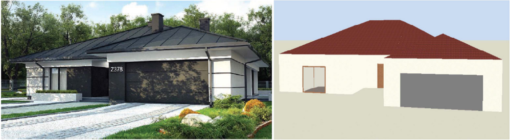
Fig. 13. Visualization of the 2010 building from the design project (left) and modeled with Design Builder software (right).
