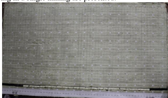
Fig.2 Deformation and failure characteristics of overlying strata with 95% filling rate
