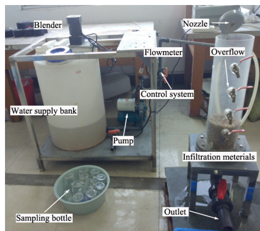
Figure 2. The device of infiltration test
