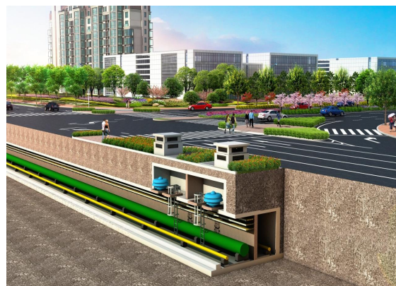
Figure 2. The Work model of underground integrated pipe gallery.
