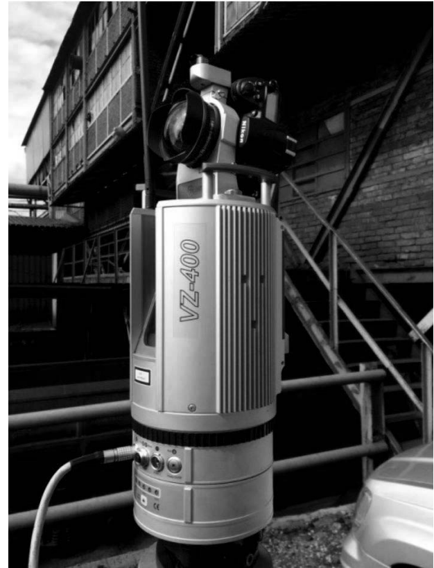
Fig. 8. 3D laser scanner Riegl VZ-400.
