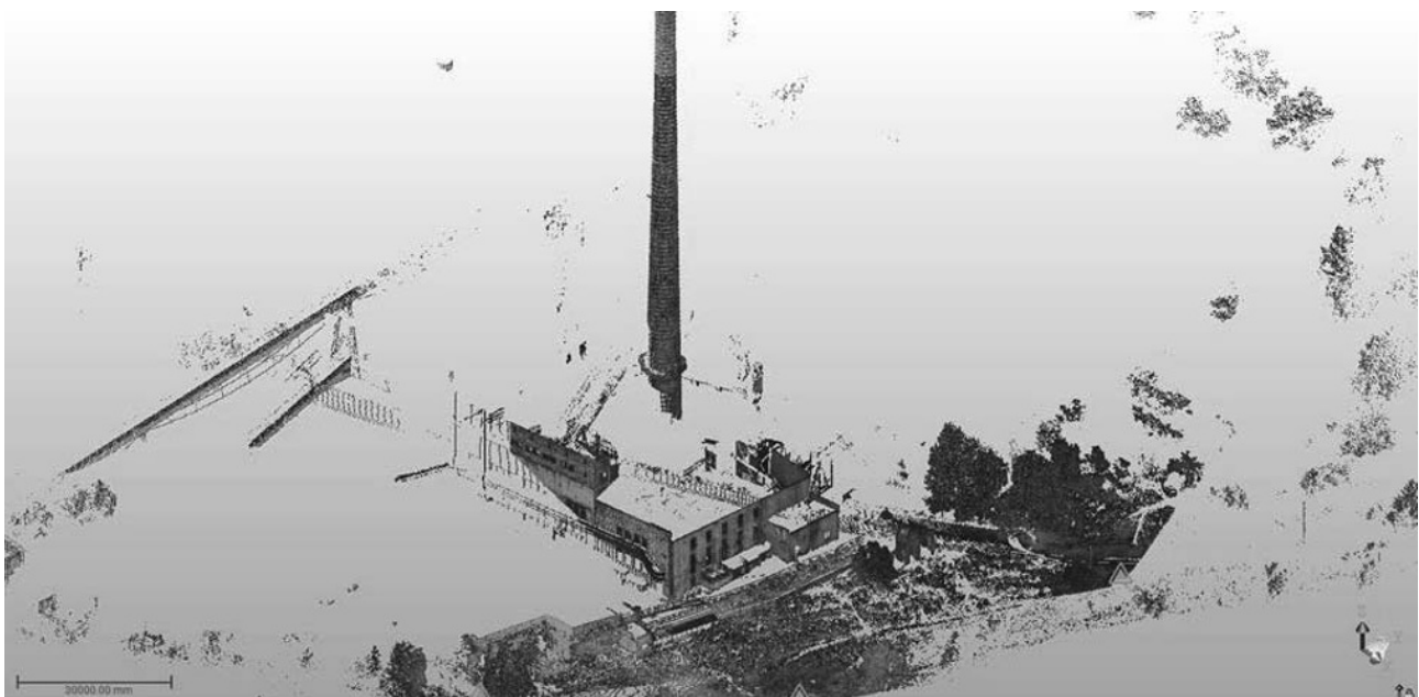
Fig. 11. Registered cloud of points and model of Terma-Dom chimney.
