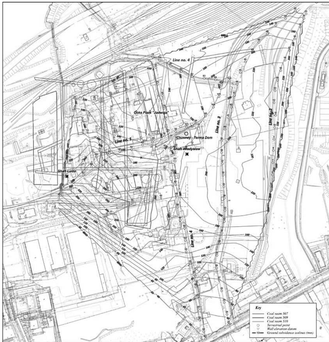
Fig. 10. Extraction of panels and headings in seams 507, 509 and 510 with subsidence contours.
