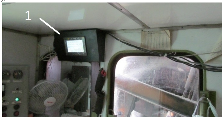
Fig. 1. The equipment installed in the cabin of the drilling rig SBSH-250MNA-32: 1- controller.
