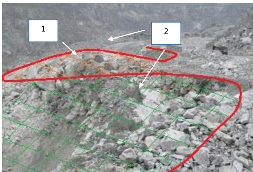
Fig. 6. Experimental site after explosion: 1-unprocessed area of diorite; 2- destroyed area of the local massif
