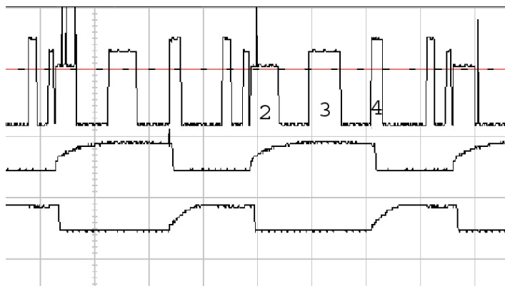
Fig. 4. Operating mode of the electromagnetic hammer No. 3 (100A, S4).
