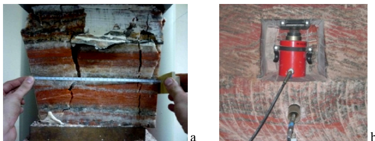
Fig.4. Determining the salt rocks modulus of deformation in laboratory (a) and field conditions (b)
