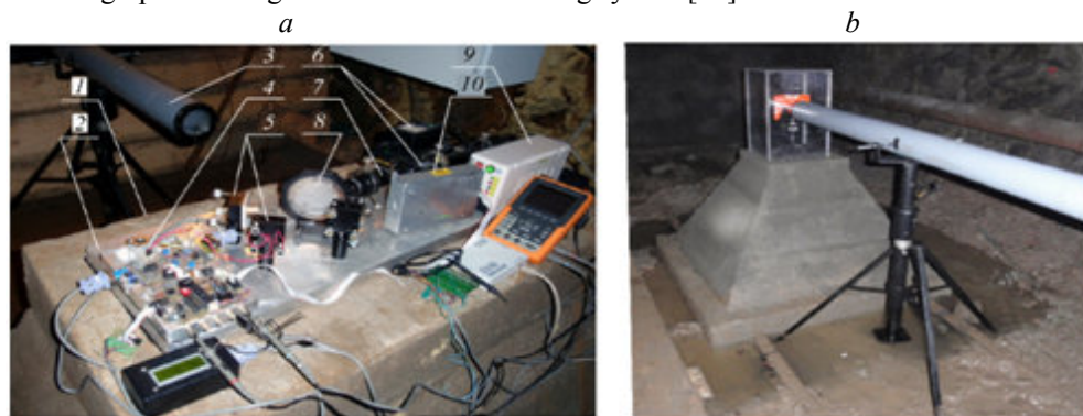
Fig. 1. Laser deformograph installed at geo-dynamic testing area in the vicinity of “Streltsovskoe” ore field: a — interferential unit; b — angle reflector and a fragment of air-filled beam mode guide: 1 — concrete bed; 2 — optical bench; 3 — beam mode guide; 4 — monitoring system; 5 — piezoceramic units; 6 — laser with a power unit; 7 — collimator; 8 — separating plate; 9 — monitoring system power unit; 10 — resonance amplifier.
