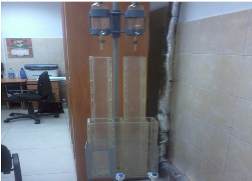
Fig. 1. A bench for geotechnological testing of ores using standard and activation schemes of percolation leaching
