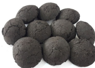
Fig. 3. Briquettes of coal underburning, made on a roll press
