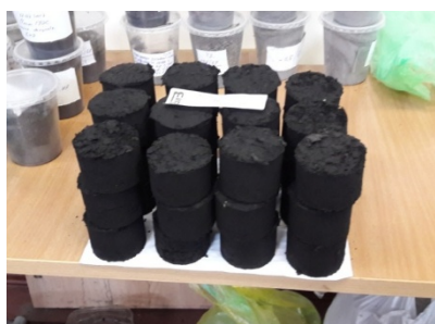
Fig. 2. Briquettes of coal underburning, made on a screw press
