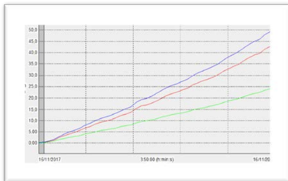
Fig. 12. Energy consumption curve chiller TAE EVO 161.
