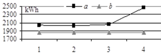
Fig. 9. Comparison of aggregate weekly power losses in the distribution network: a – for three options with permanent configuration; 1-3 and 4 – under the lack of reconfiguration; b – at optimum hourly reconfiguration
