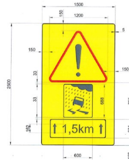
Fig. 1. Experimental signage to "inform about deteriorated conditions during rainfall"
