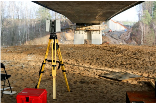
Fig. 10. Laser scanner Leica P30 station.
