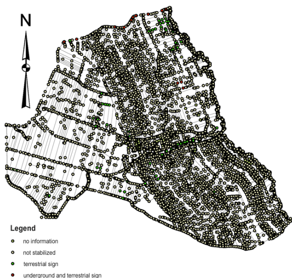
Fig. 9. The values of the border point stabilization code in Żelazówka, source: own study.
