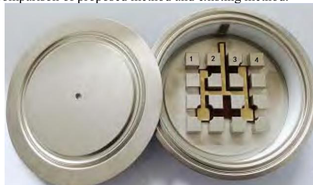
Fig. 4. Copper emitter pillars layout of press-pack IGBT
