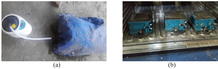
Fig. 1. (a) Portable steam curing, (b) Oven curing
