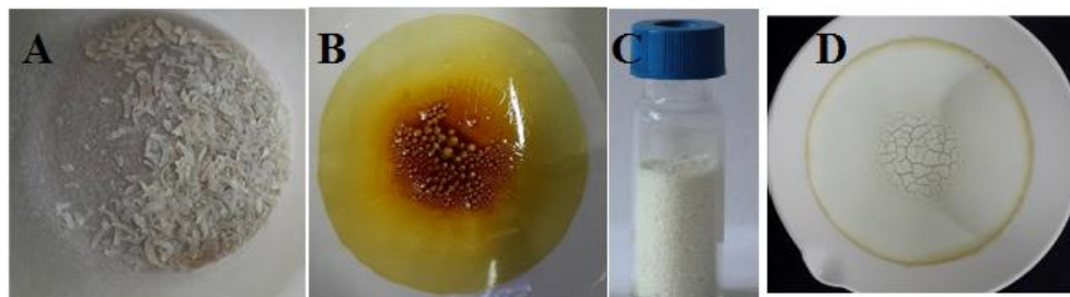
Fig. 1. Image of (A) human fingernail, (B) solid CQDs, (C) pure g-C 3 N 4 and (D) CQD/g-C 3 N 4 .
