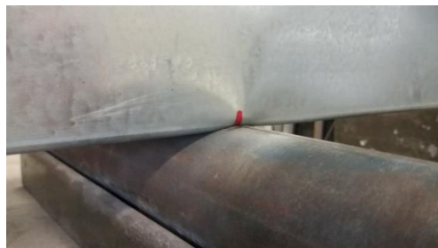
Fig. 10(a). Local buckling of bottom chord for conventional truss specimen.
