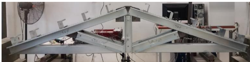
Fig. 6. Conventional CFS roof truss specimen.
