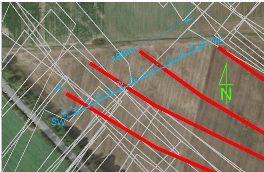
Fig. 6. Location of ERT profile (blue) on the background extracted fields edges (gray) and the course of linear deformations (red).
