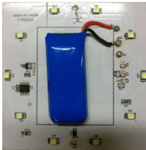
Fig. 2. Bottom view of the solar emergency lamp circuit
