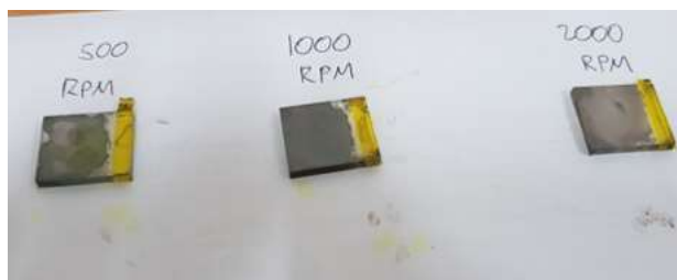
Fig 9. The condition of device after MAPbI 3 deposition.
