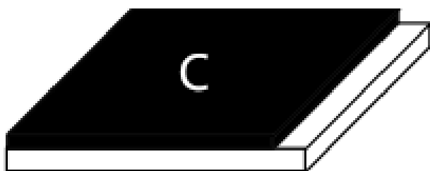
Fig 6. Carbon Powder deposit procedure on a FTO glass plate, covering 3/4 of its surface.
