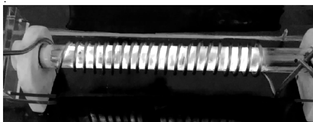
Fig. 4. Dielectric barrier discharge (DBD) reactor used in the experimental study.
