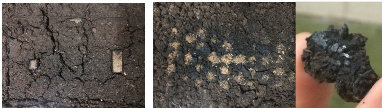
Fig. 7. Rewetted peat after the rewetting experiment. MC 90% (left), MC 60% (right)
