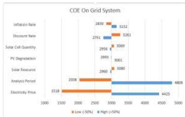
Fig. 14. Tornado Chart of LCOE (On Grid)
