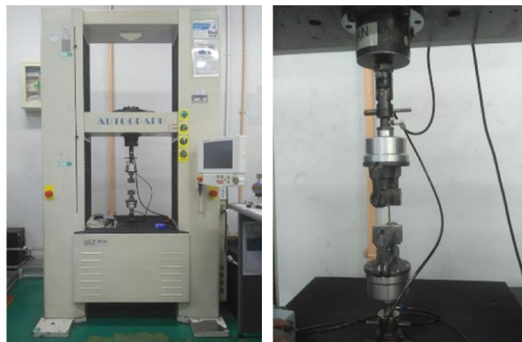
Fig. 10. Placing in the clamps of the Shimadzu AG-IS 20 kN Machine unit (left) Clamps (right)
