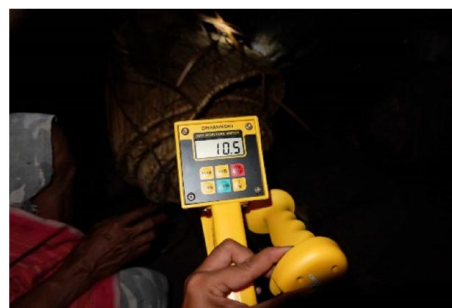
Fig. 5. Measuring material humidity at lobo using Draminski HMM
