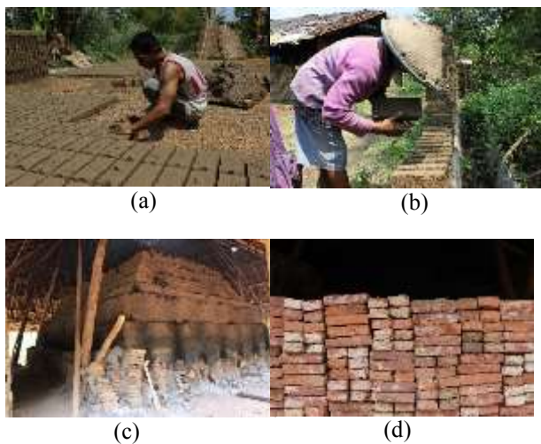
Fig. 2. Traditional brick making process in Pedurungan Kidul
