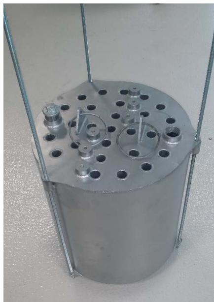
Fig. 8. PCM based insert for thermal energy storage tank.
