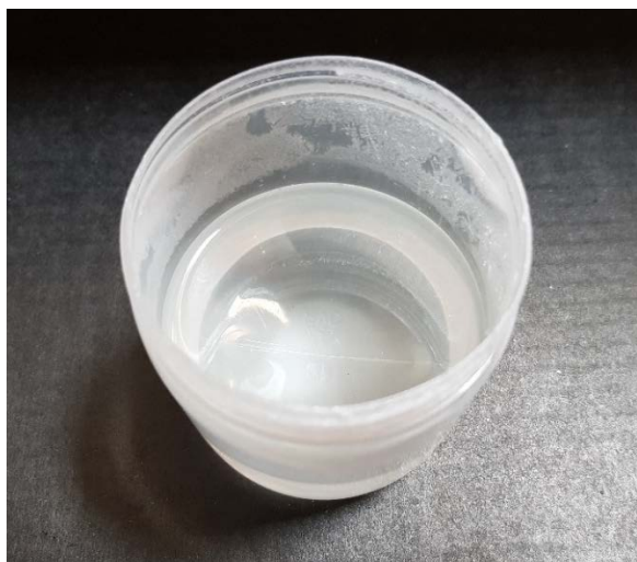
Fig. 3. CrodaTherm53 after melting – liquid phase.
