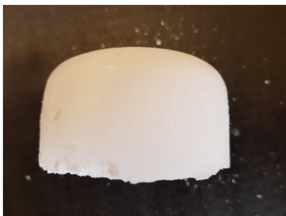
Fig. 4. CrodaTherm53 after re-solidification – solid phase.
