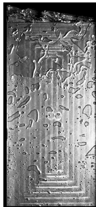
Fig. 9. The development of flow boiling on a vertically oriented plate of minigap evaporator (minigap thickness = 1 \text{ mm} ); visible flow structures (from the bottom to top): bubbly, slug and churn.
