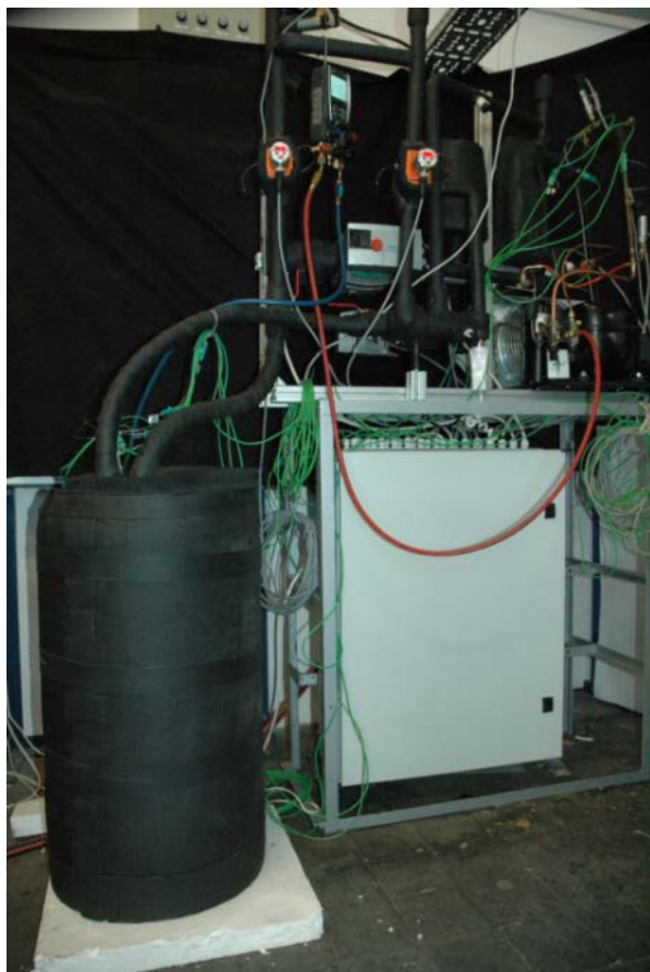
Fig. 3. Photo of the stand dedicated to investigation of the dynamic characteristics of LTES.
