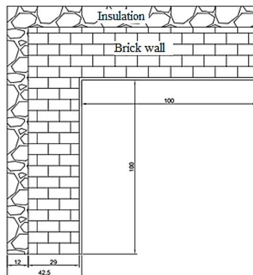
**Fig. 4.** Geometrical model (all dimensions are in cm).
