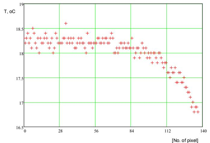
**Fig. 3.** Wall surface temperature along the line L1.
