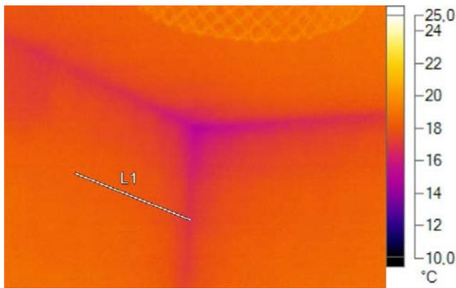
**Fig.1.** Thermal image of the structural thermal bridge.
