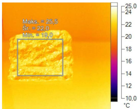
**Fig. 2.** Evaluation of the reflected temperature.
