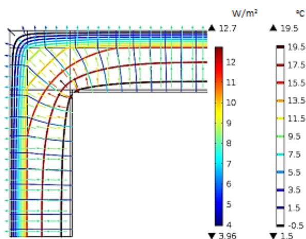
**Fig. 5.** Streamlines, temperature and heat flux in the wall corner.
