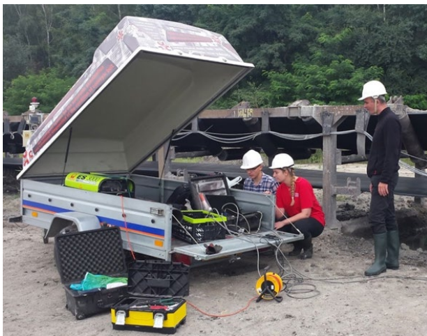
Fig. 1. The DiagBelt system during tests on a belt conveyor in an open pit mine.
