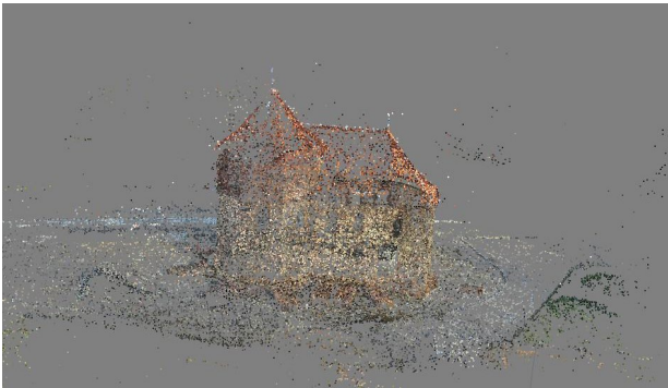
Fig. 2. Distribution of tie points used in bundle adjustment (sparse point cloud) of St. Martin Church in Wrocław model.
