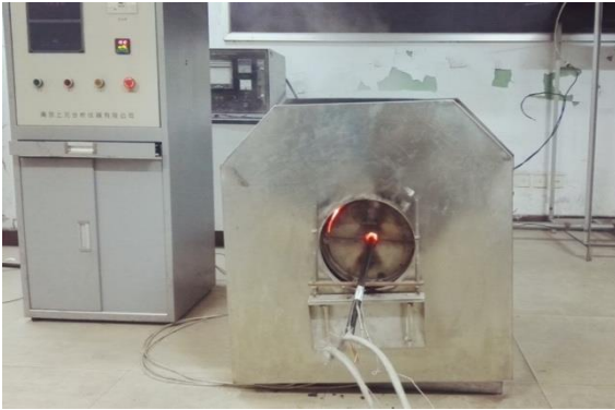
Fig. 6. SDR-1 cable thermal radiation experimental furnace.
