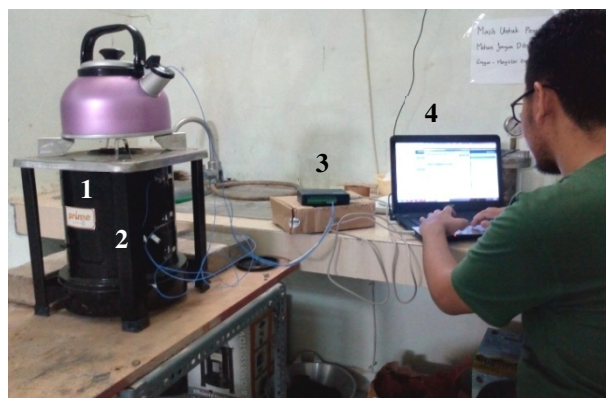
Fig.1. Experiment of the waste heat recovery system study in the wooden cooking stove using TEGs.
