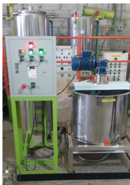
Fig 2 Photo Granulator Vacuum with capacity of 50 kg / day
