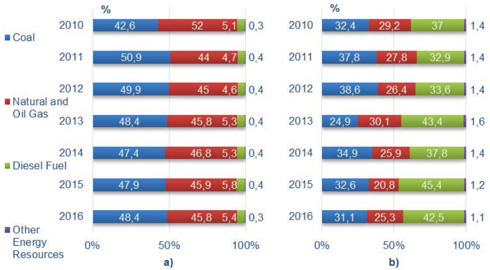
Fig. 2. Comparison of the structure of fuel consumption for the electricity generation in power stations of Sakha Republic in physical (a) and value (b) terms
