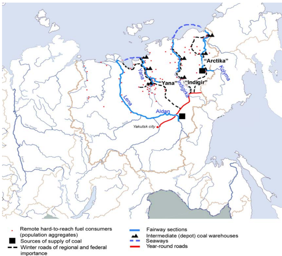
Fig.2 The main transport corridors (waterways and winter roads of regional importance) supply of remote hard-to-reach consumers of the Republic of Sakha (Yakutia).
