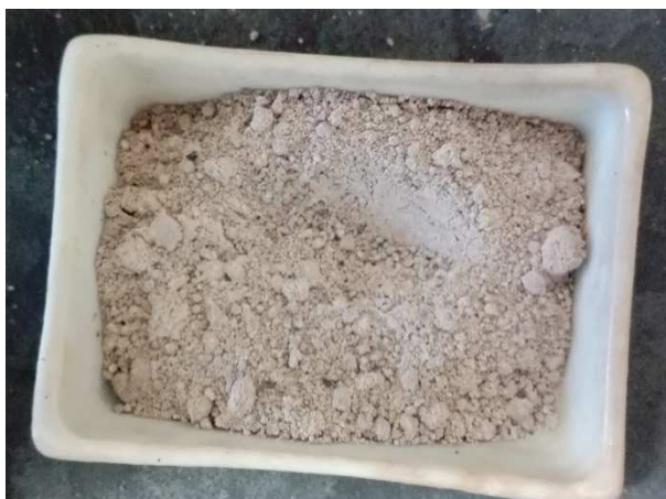
Fig. 2. Sample decomposed in 900°C – ratio 5
