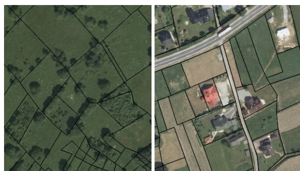
Fig. 1. Actual manner of land development and parcel boundaries A) No correlation B) Strong correlation
