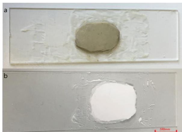
Fig. 1. Prepared clay samples on glass slide; a) bentonite b) kaolin (samples are approximately 20 mm in diameter).
