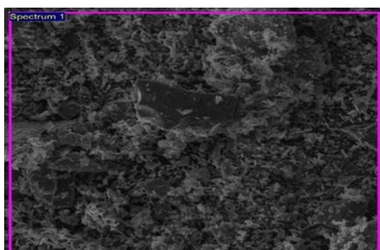
Fig. 2. SEM of gold tailings before leaching
