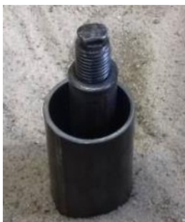
Fig. 7. A perch screwed to pile base
