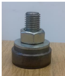
Fig. 6. Steel bottom of pile model.
