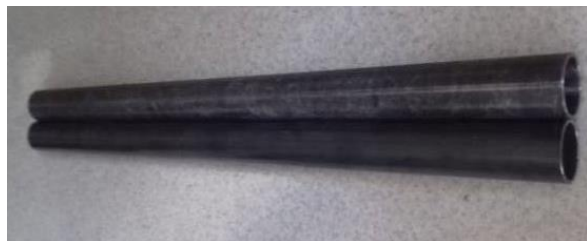
Fig. 5. Steel pipes with 40 mm external diameter
