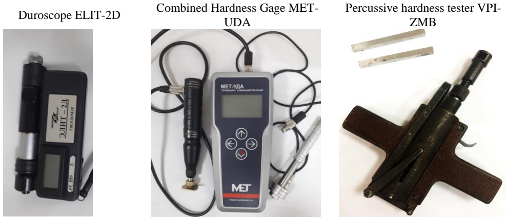
Fig. 3. Devices for determining the mechanical properties of steel by the methods of hardness testing
