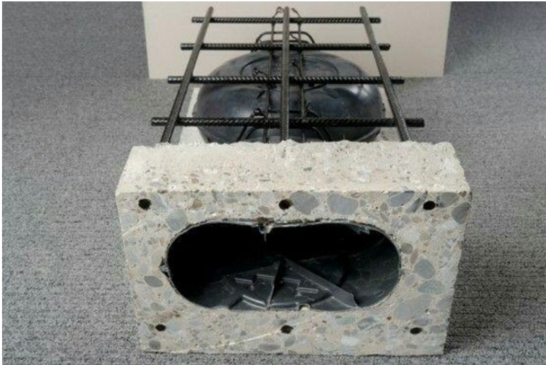
Fig. 1. Fragment of a slab with a void formers Cobiax
