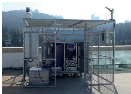
Figure 1. Measurement site with multiwavelength lidar Polly XT at the rooftop of the Electrical Engineering building of Technion.
