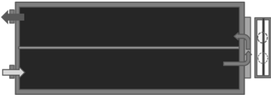
Fig. 5. Schematic diagram of the collector and airflow inside the collector.
