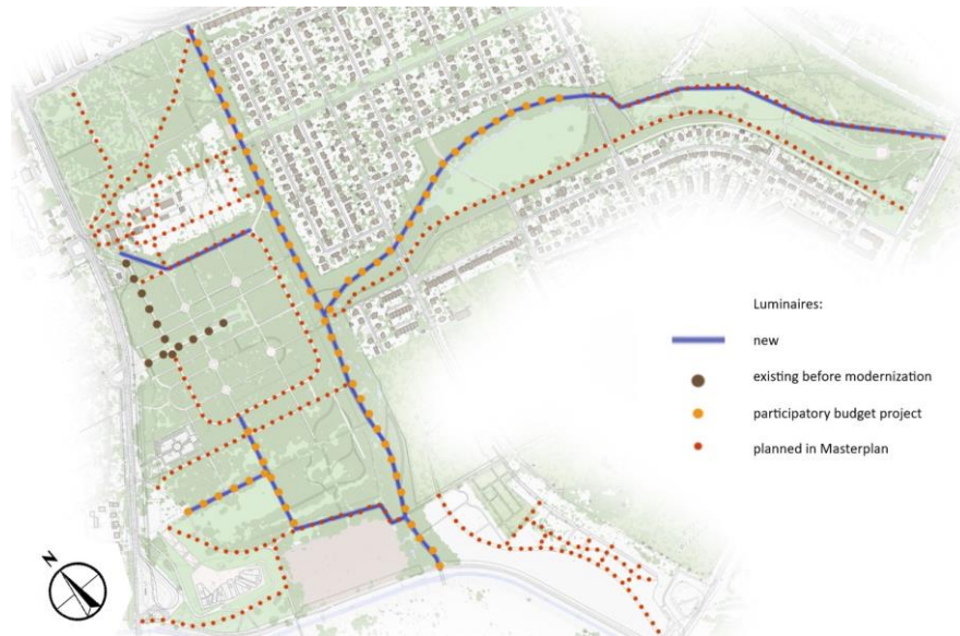
Fig. 2. The brown dots show existing lamps, orange dots represent winning participatory budget project and the smallest red ones lamps planned in Masterplan [20]. Spatial distribution of the new luminaires is indicated by the blue line [graphic based on ZZM Wrocław data].
