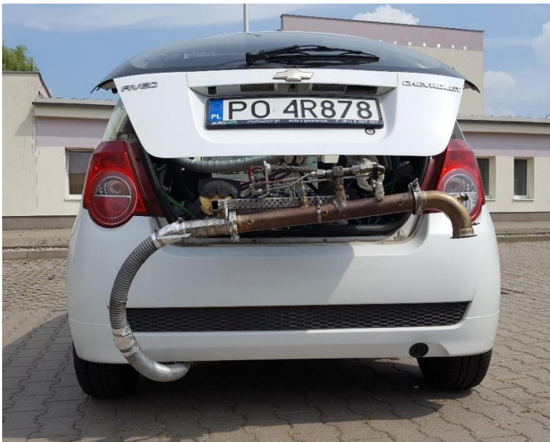
Fig. 3. The SEMTECH DS measurement equipment with the flowmeter mounted on the vehicle.
